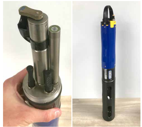
Prepare the EXO Sonde by installing the Turbidity Sensor as well as the probe guard.
